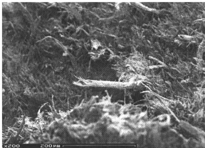
FIGURE 3 Fracture surface appearance and material microstructure of Zelfo HZ
